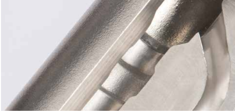
Figure 12 - Close-up of side channel finished with AFM
