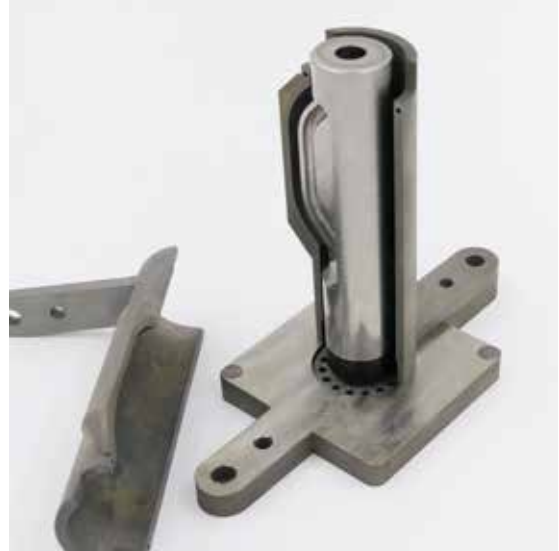
Figure 11 - COOLPULSE tooling showing cathode and part
